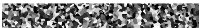
FIG. 2. An example of a nanowire with dimensions 200 \text{ nm} \times 1600 \text{ nm} subdivided into Voronoi cells (grayscale) with average diameter 20 nm.
