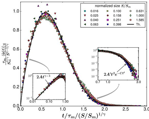
FIG. 5. Scaling collapse of the average shape at fixed avalanche sizes  $\langle \dot{u}(t) \rangle_S$ , according to Eq. (7), in the FeSiB thin film. The continuous line is the prediction for the universal SR scaling function of Eq. (9). The insets show comparisons of the tails of the data with the predicted asymptotic behaviors of Eqs. (10) and (11), setting  $\epsilon = 2$ , with  $A = 1.094$ ,  $A' = 1.1$ ,  $\beta = 0.89$ ,  $C = 1.15$ , and  $\delta = 2.22$ .
