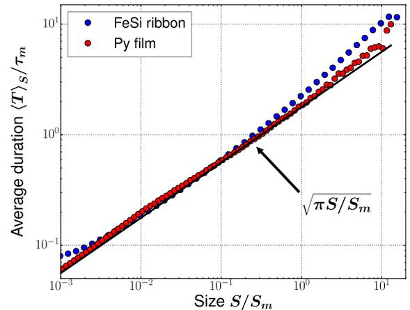
FIG. 3. Normalized average duration  $\langle T \rangle_S / \tau_m$  of avalanches in the FeSi ribbon (blue dots) and the Py thin film (red dots) as a function of the normalized size  $S / S_m$ . The continuous line is the theoretical prediction of Eq. (6).
