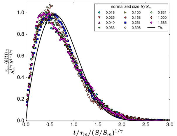
FIG. 6. Scaling collapse of the average shape at fixed avalanche sizes  $\langle \dot{u}(t) \rangle_S$  in the FeCoB ribbon using the theoretical values of  $\gamma$  and  $\tau_m$ , as in Fig. 2. The collapse deviates from the universal functions predicted for SR systems (continuous black line) in the absence of eddy currents.
